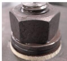
Figure 12 – Assembly with two hardened washers
