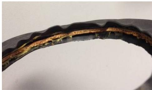
Figure 9 – Sample of CE + CR after test
