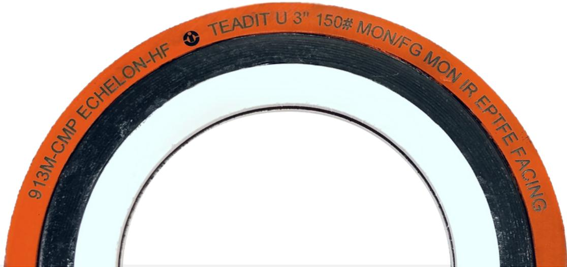
Specifically designed for Hydrofluoric Acid (HF), to safely seal an extremely dangerous chemical, as well as where crevice corrosion is a concern, Teadit®'s Echelon-HF™ Gasket is a superior choice. This design is based on an ASME B16.20 spiral wound (primary seal), but with a camprofiled Monel® inner ring, providing all the advantages of an inner ring and thick ePTFE facing materials with the added benefit of creating a secondary seal that extends further towards the bore of the pipe.
